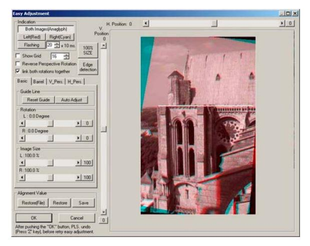
The most common, useful adjustments are the slider bars at the top for H. POSITION and the middle slider for V. POSITION.
